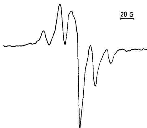
Figure 3. ESR spectrum of 3,4-PI adsorbed on silicagel irradiated and measured at -196^{\circ} , dose 6.2 \times 10^{19} eV/g.
